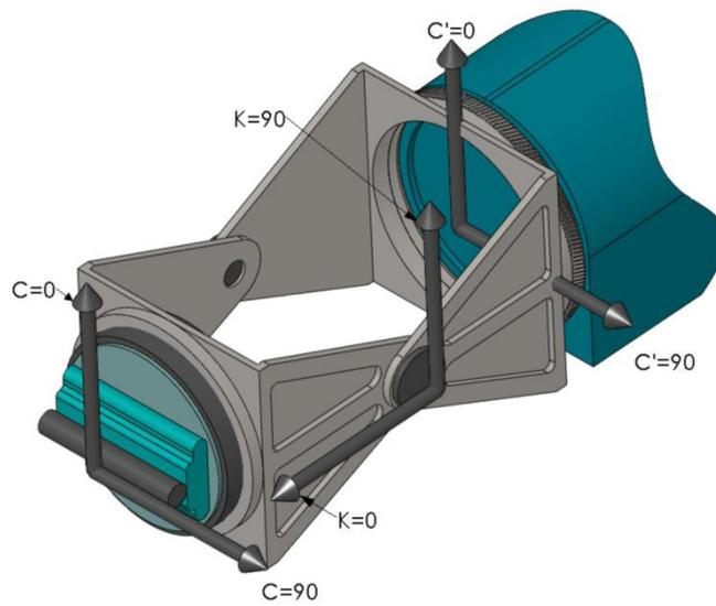
Figure 6. C'KC axis arrangement
