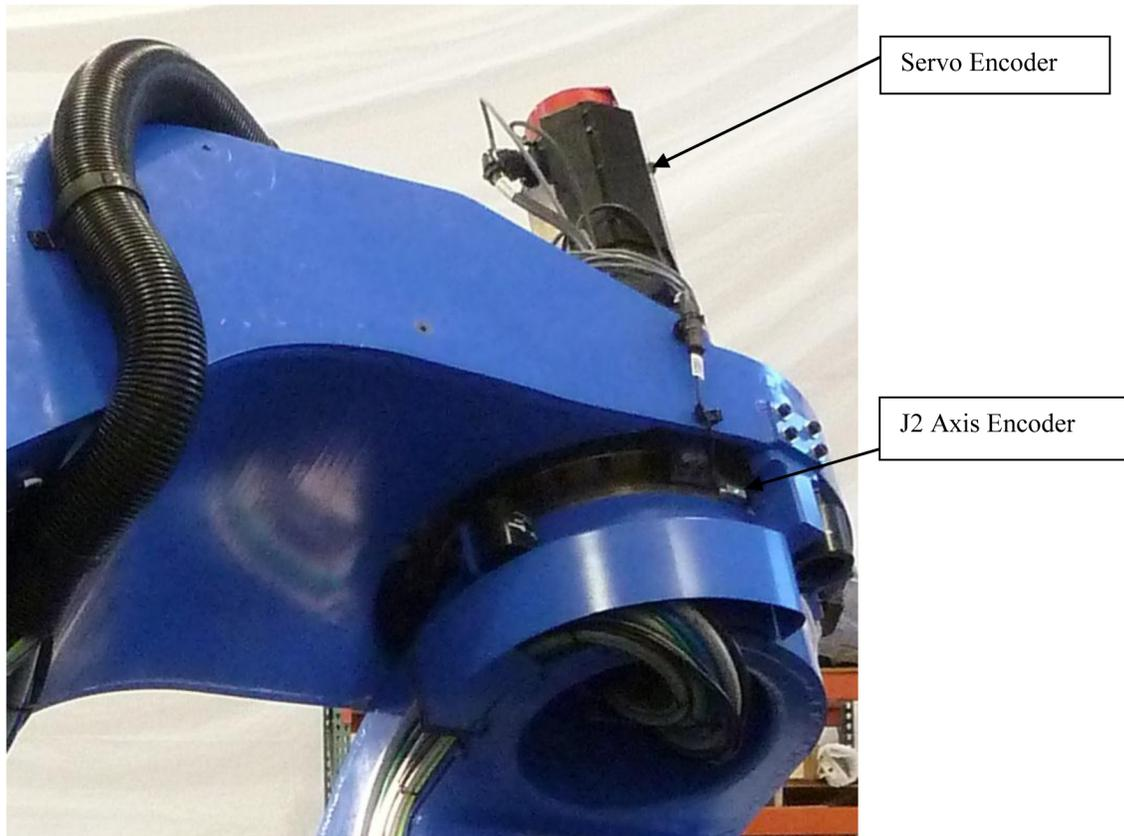
Figure 8. Servo encoder and axis encoder locations.
