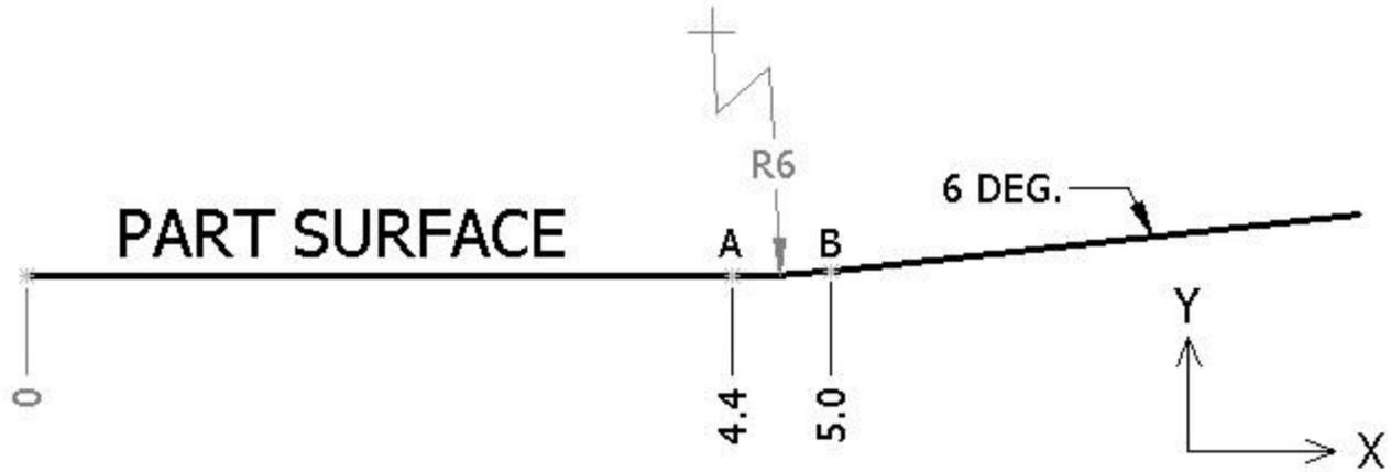
Figure 3. Small 6-degree ramp on part surface.
