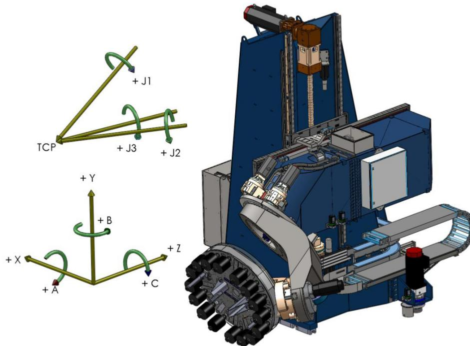
Figure 5. Naming convention for non-orthogonal axes.
