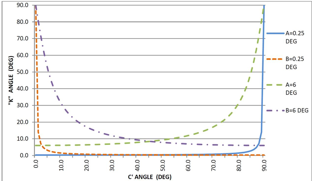
Figure 7. K and C' angles for constant A and B axis angles.
