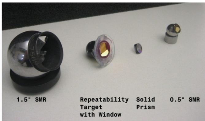
*Figure 1. Laser Tracker Target for Comparison*
