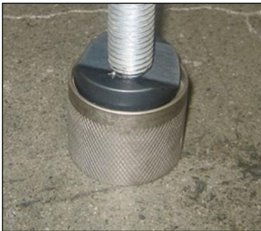
Figure 8. V-block Mounting Point (components)
