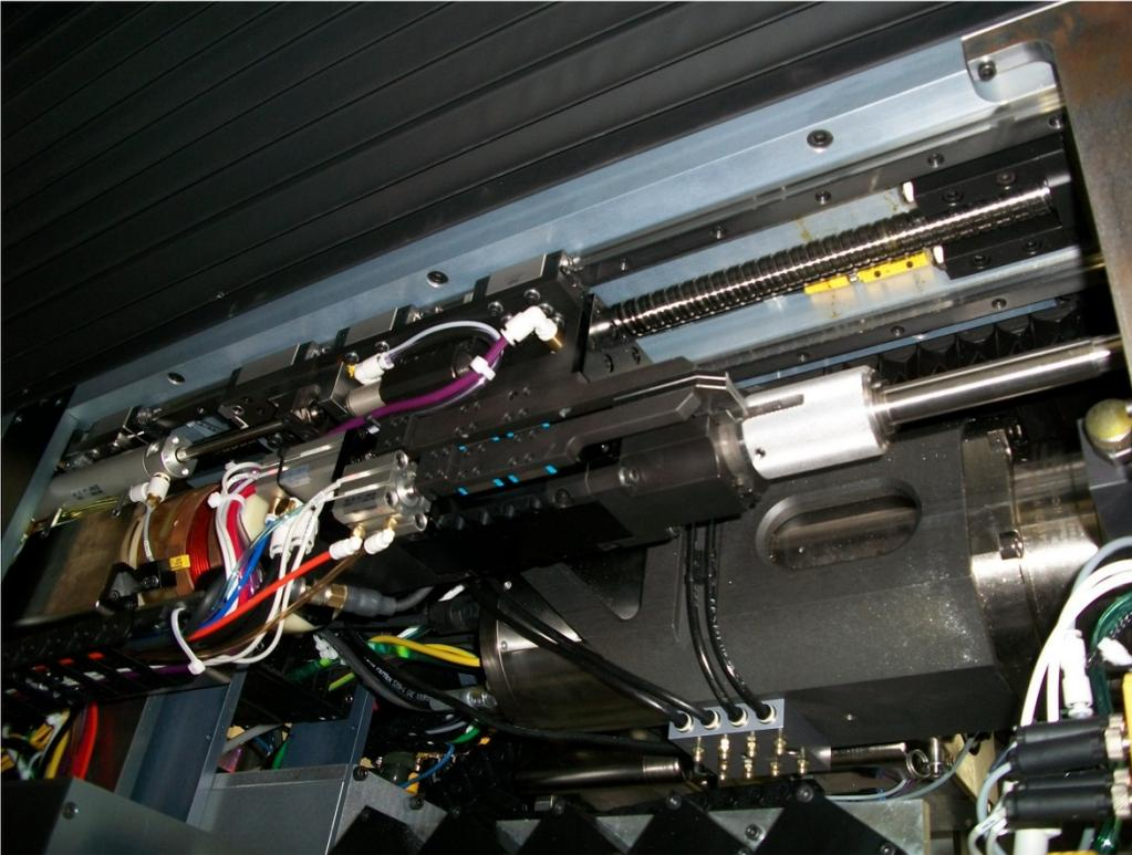
*Figure 1 The EMB mounted on the riveting machine*
