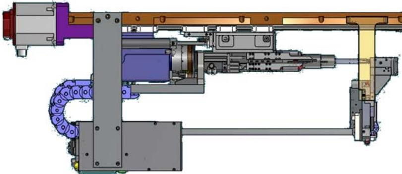
***Figure 3: Injector receives the bolt and delivers the bolt to the collet fingers***
