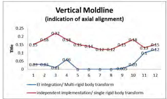
**Figure 2.** The above data shows the measured deviation of a mostly vertical (actually circumferential) line projected on a matching machined line on the part surface. This is an indication of the axial alignment of the laser projection to the mandrel.
