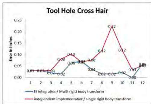
**Figure 1.** The above data shows the measured deviation of the projected cross-hair to the center of the hard tooling-hole location. This is largely in-line with our expectations based on the data gathered during probing.
