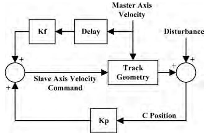
**Figure 5. Block diagram of the control loop for continuous C-squaring, with feedback gain given by  $K_p$**
