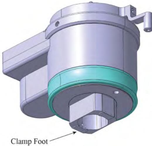
**Figure 4. Nosepiece with gimballed clamp foot.**
