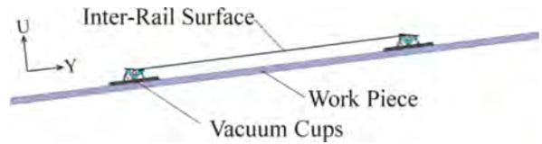
Figure 3. Cross section of the inter-rail surface, looking along the direction of the X axis.
