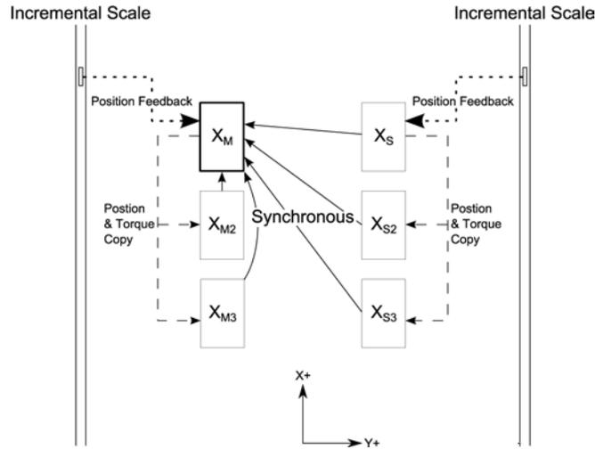
Figure 7. X-axis Controls Configuration
