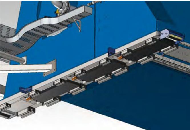
**Figure 6. Multiple linear motors are used on the same axis to improve machine top speed and acceleration.**
