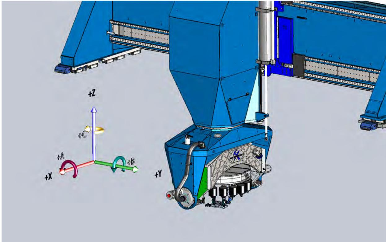
*Figure 11. Machine axis coordinates.*
