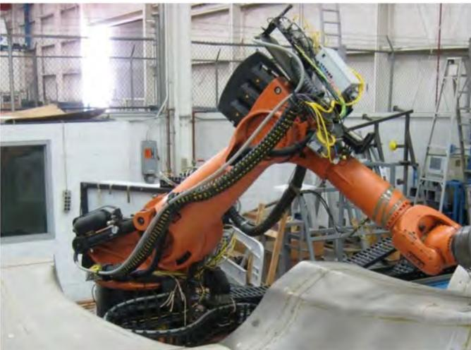
**Figure 1. KUKA KR 500 L480-2 MT laboratory robot**
