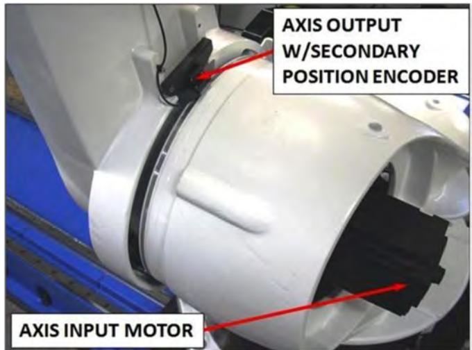
**Figure 2. Secondary encoder mounted to output of a robot axis (KR500 shown)**
