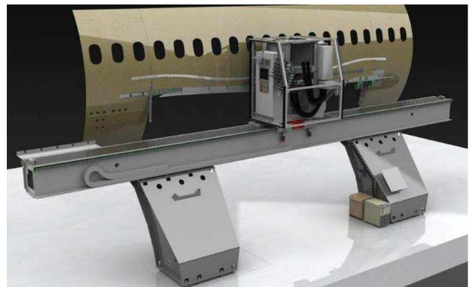
*Figure 1 Side-of-Body Drilling Machine*
