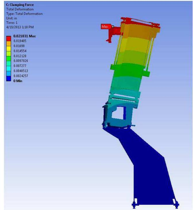
Figure 9 Machine Deflection under 1200# Clamp Load
