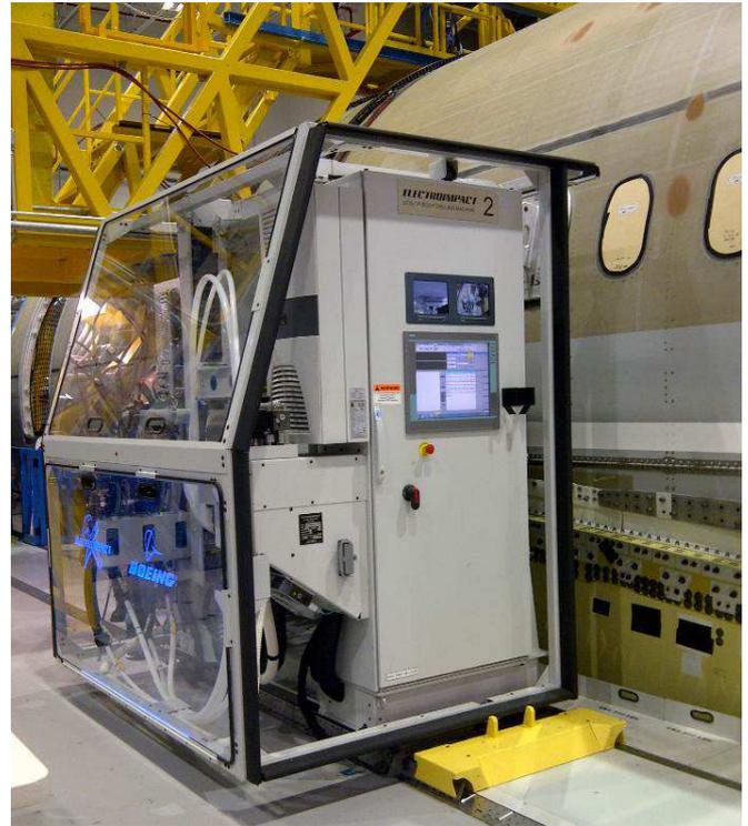
*Figure 16 Side-of-Body Drilling Machine*
