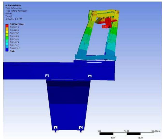
Figure 10 Machine Deflection under Shuttle Load
