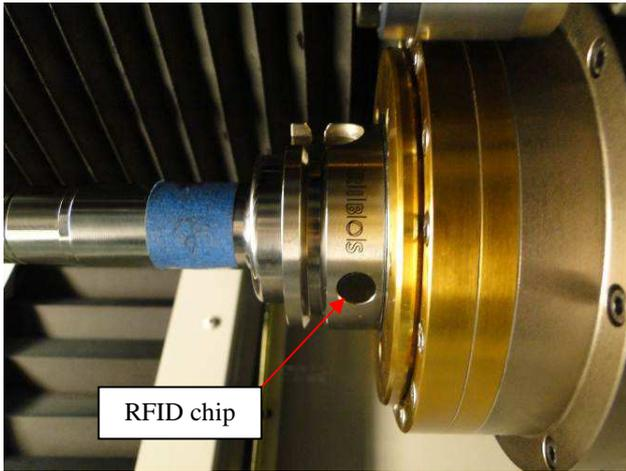
*Figure 12 RFID Chip*
