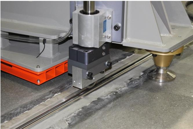
*Figure 13 Air Caster and Strothmann Rail*
