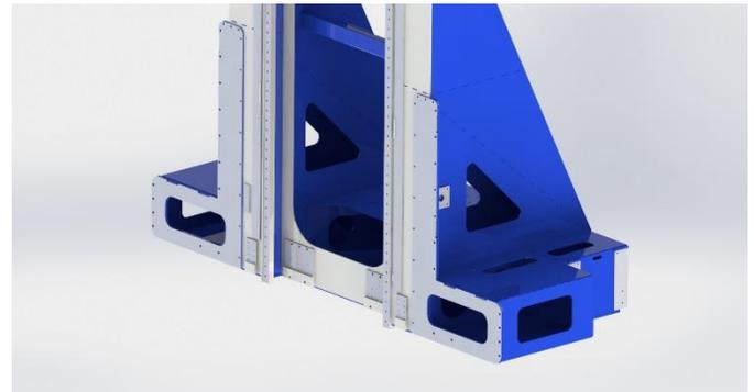
Figure 12: Side bolster and platform deck are designed to be a structural plinth and mounting surface, with good access from top and sides
