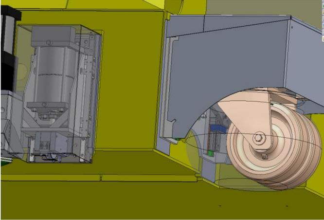
*Figure 13: Pneumatically deployed Strothmann wheel for rail guidance, mounted near lifting caster*
