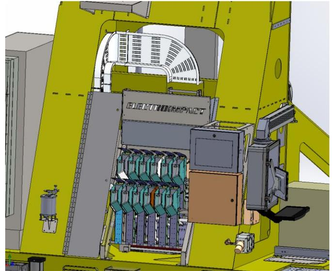
Figure 11: Routing of wireway allows freedom to place equipment, and access to equipment from both sides when it is in place
