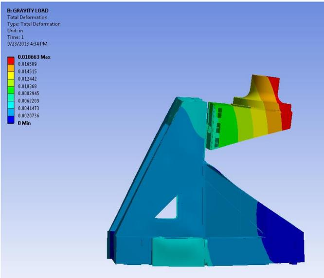
Figure 5: Sled at top of stroke: overall toolpoint deflection 0.034"
