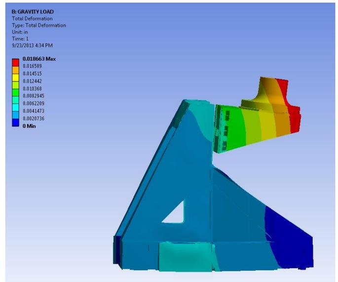
Figure 8: The Y sled was analyzed as part of the system with the frame and the robot base
