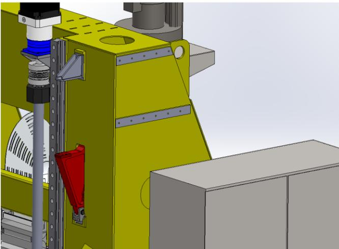
*Figure 14: Hardstop/Flag indicating the Y axis is locked out; usually the Y sled would be positioned above the moving hardstop when the hardstop is extended*
