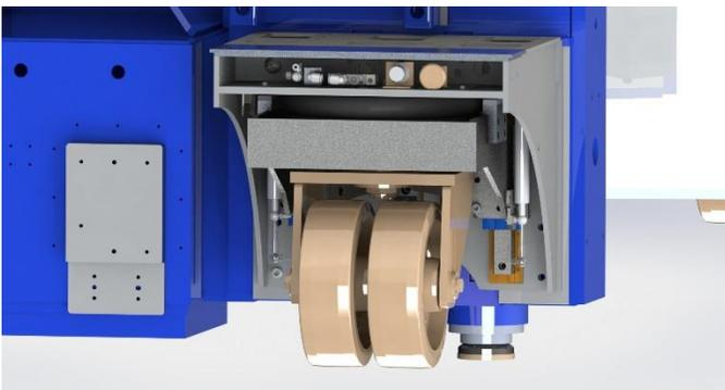
Figure 10: pneumatically deployed caster with rigid mount swivel foot in background
