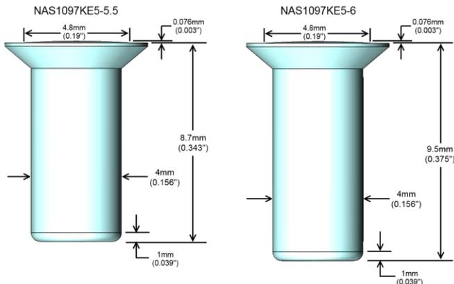
Figure 1. NAS1097KE5 rivets with dimensions.
