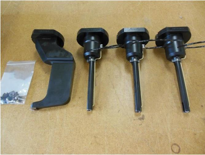
Figure 4. Range of lower anvil tooling.
