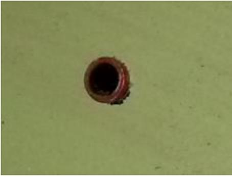
Figure 13. Cherry tack rivet used for resynching installed in panel.
