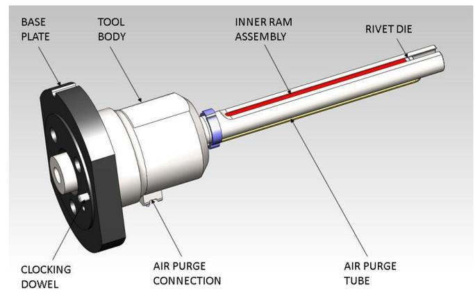
Figure 3. Lower tubular clamp inside riveting anvil.
