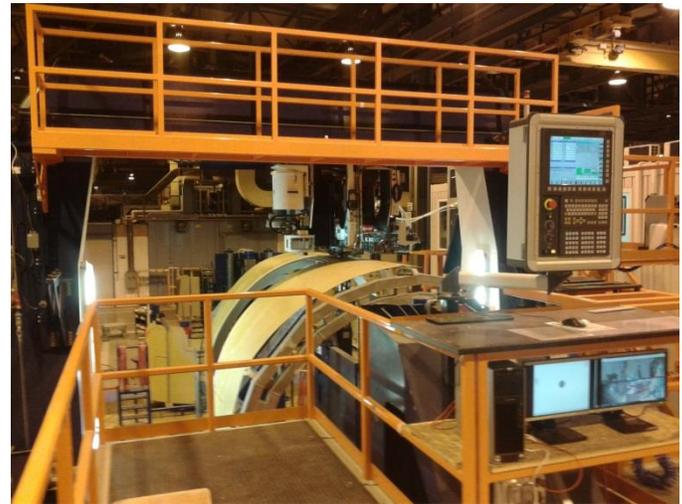
Figure 11. E7000 machine with an A320 side panel loaded.
