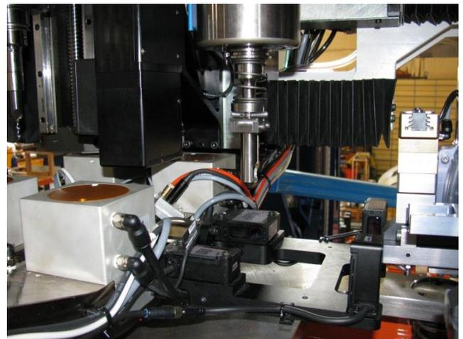
Figure 9. Upper anvil and fingers above two of the four clamp cylinders.
