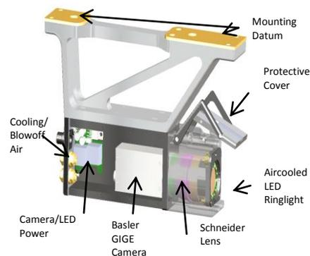
Figure 12. Internal view of the resynch camera..
