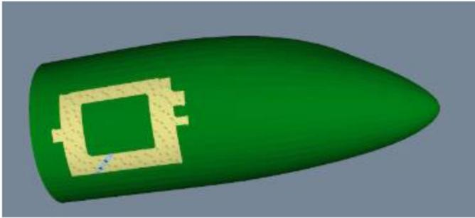
Figure 5. Operator display highlights course laser is projecting
