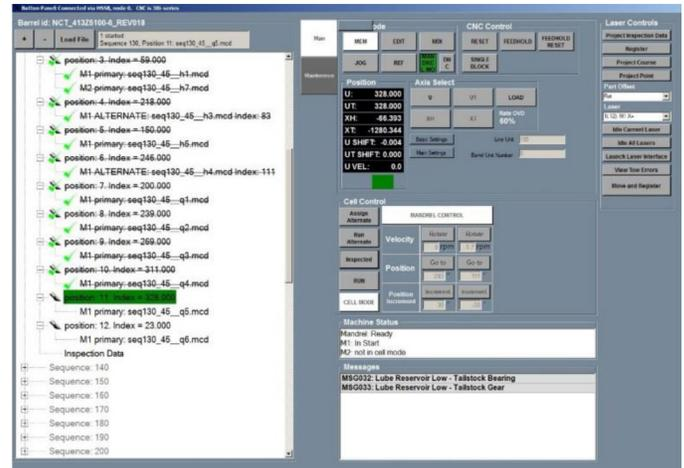
Figure 6. Part program sequence including inspection data in each sequence
