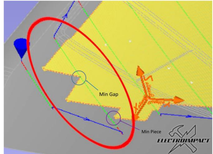
Figure 3. min gap and min piece in a layup. These occur regularly in 45 degree plys
