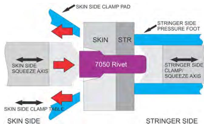
Figure 4. During the Servo/Servo move, the head is pinned into the countersink by the squeeze axis.
