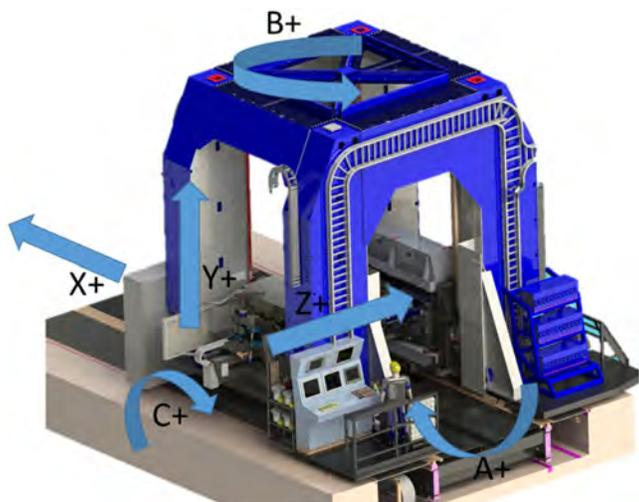
Figure 1. Vertical fastening machine overall arrangement.
