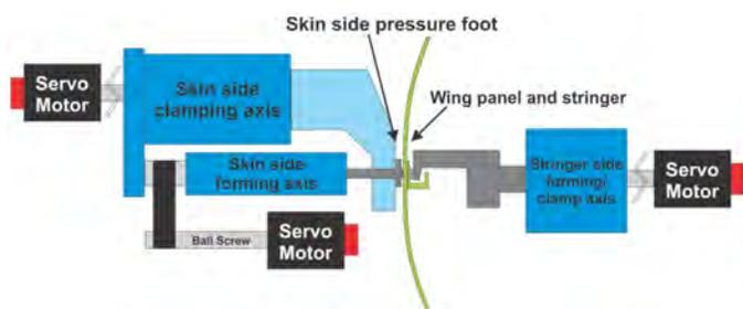
Figure 2. Mechanical upset arrangement.
