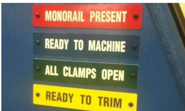
Figure 22. Placards mounted to PAL jig provide explanation of colored stack lights that work in conjunction with control interlocks.
