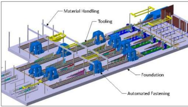
Figure 2 Panel Assembly Line (PAL) Subsystems.
