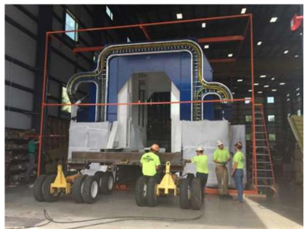
*Figure 10 Transport dollies are mounted prior to departure. The orange frame is added and covered in shrink wrap to protect the machine for the duration of the trip.*
