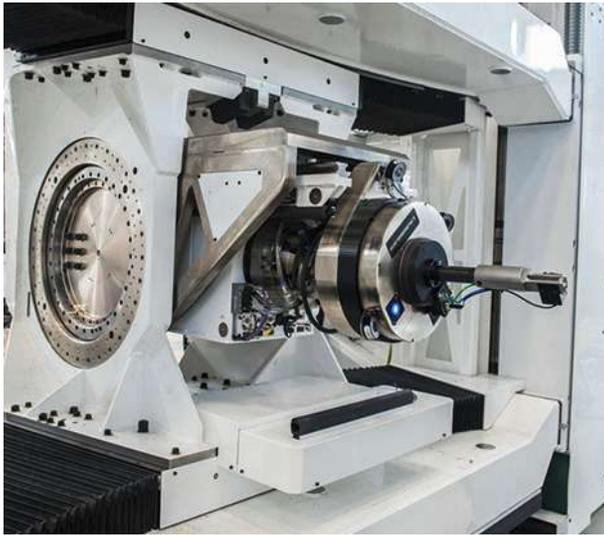
*Figure 13 Rivet forming process head, V-side.*
