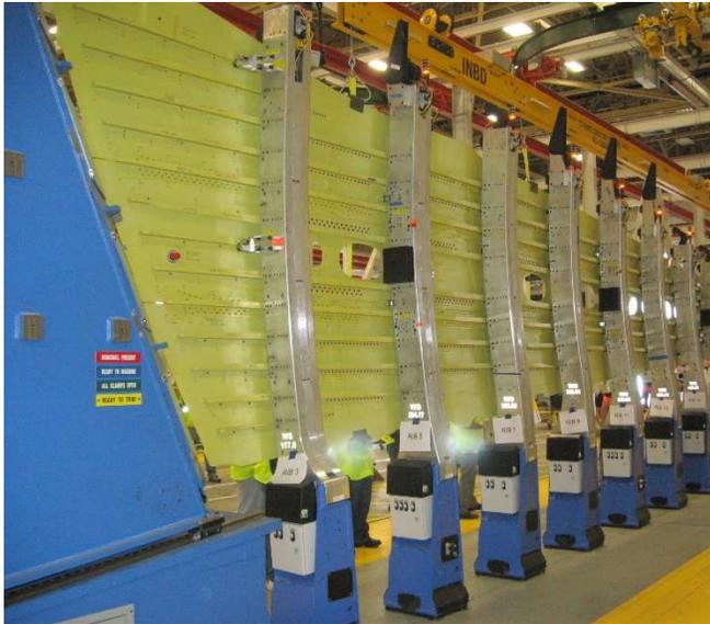
*Figure 16 Tooling posts were placed in complementary positions from one cell to the next to avoid manipulating the tool during production.*
