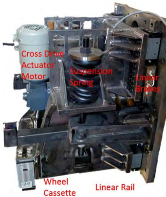
Figure 7. Wheel System Prototype Details - View from Above
