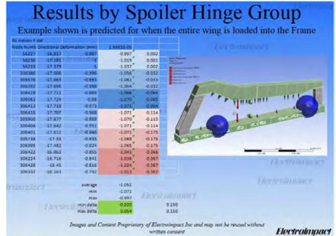
Figure 9. Example of Deflection Predictions for a Live Load
