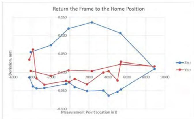
Figure 13. Measured index points of repeatability following a frame move 5m in X and returned to the home position.
