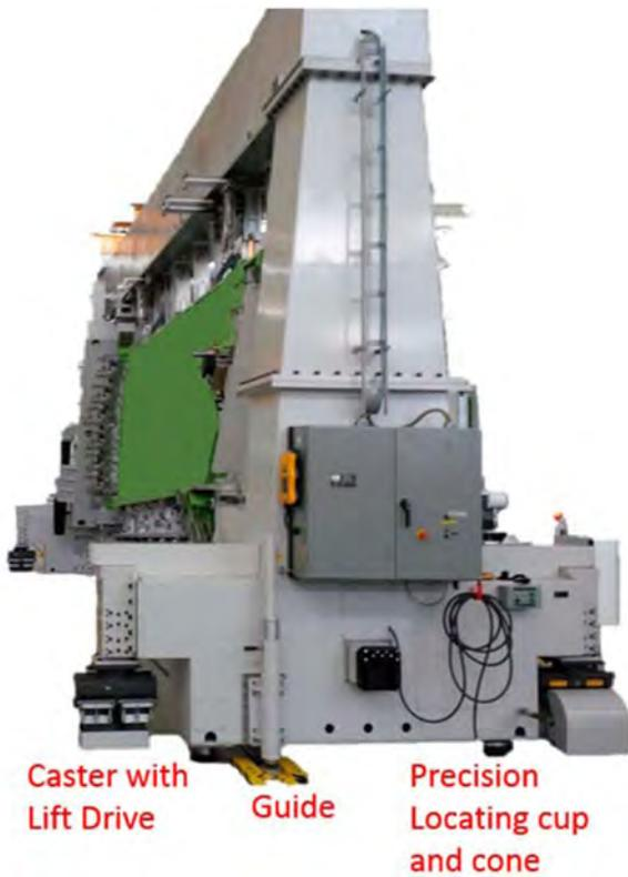
Figure 1. Alternative caster-supported system considered
