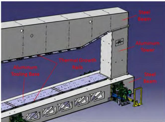
Figure 4. Thermal growth rails and fixture materials
