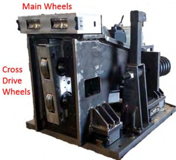
Figure 8. Wheel System Prototype Details - View from Below
