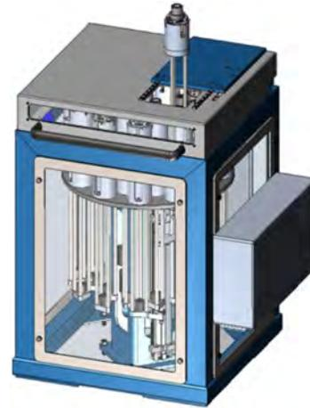
Figure 8. Automatic Tool Changer
