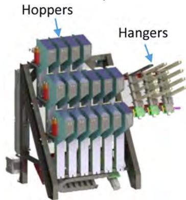
Figure 7. Fastener Feed System
