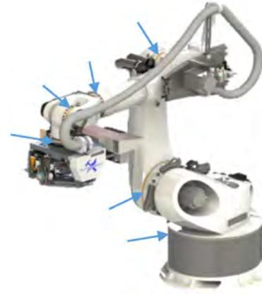
Figure 4. Accurate Robot with Arrows Pointing to External Scales on Each Axis
