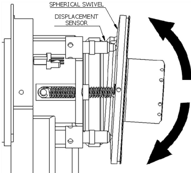
Figure 2. A spherically compliant contact pad with displacement sensors for normality feedback.
