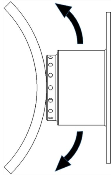
Figure 3. A compliant contact pad with a flat contact surface will wobble or cock to one side when clamped against a highly curved surface.
