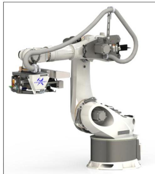
Figure 1. An articulated arm robot with secondary feedback on all axes and a multi-function end effector.
