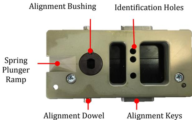
**Figure 6: Cartridge Loader Assembly**
