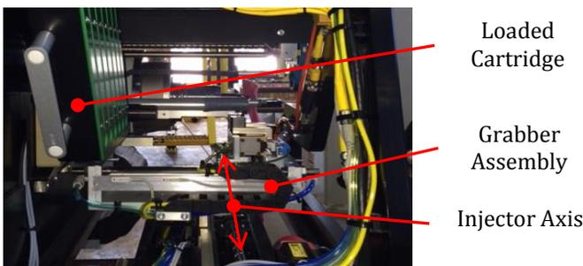
**Figure 7: Injector Assembly Components**
