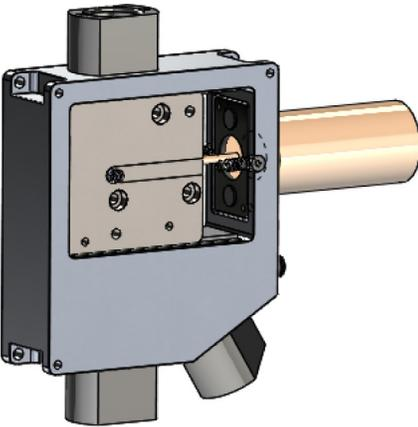
Figure 7. Fastener Eject Actuator Assembly
