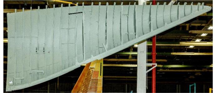
Figure 3. Right side panel of C-130J aft fuselage with structure visible, showing deep circumferential frames that must be fastened directly to the skin.
