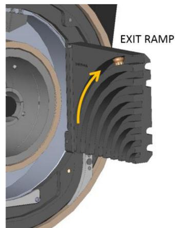
Figure 13. Fastener exiting spinner.
