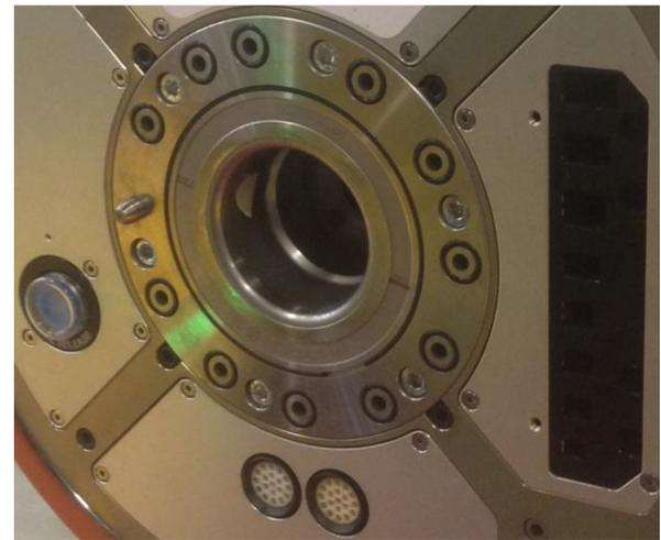
Figure 8. Automatic tool changer interface.
