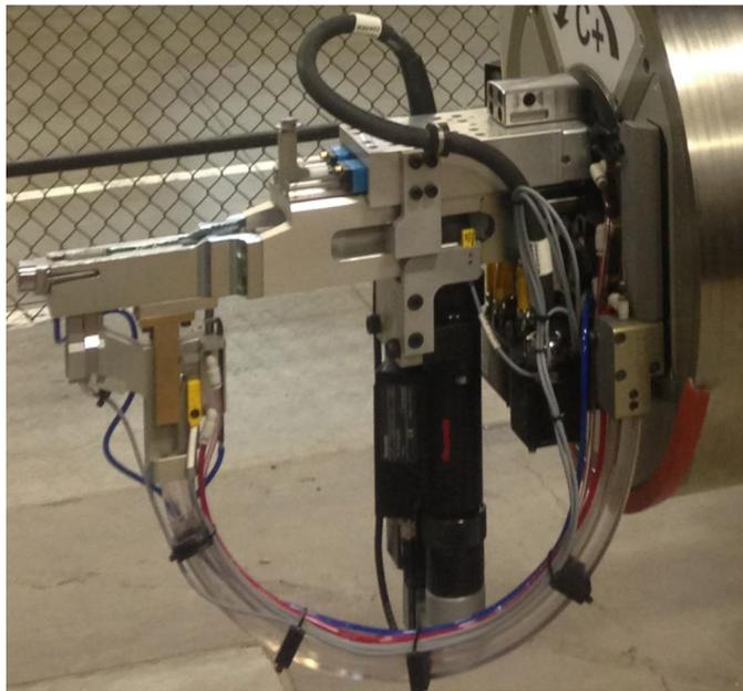
Figure 1. Wet side anvil for nut installation.
