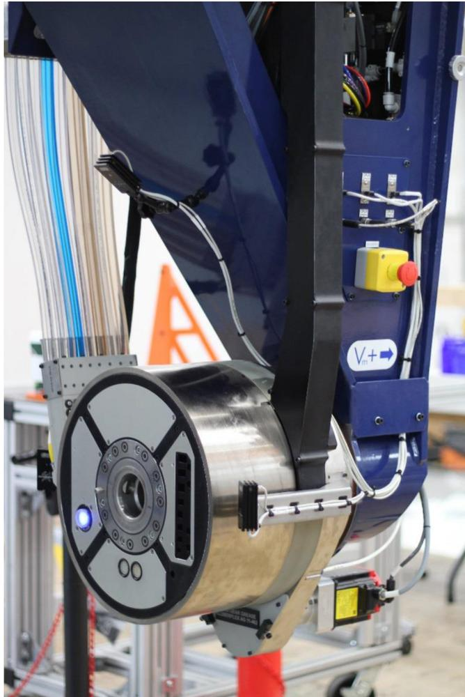
Figure 3. C Axis with spinner assembly.
