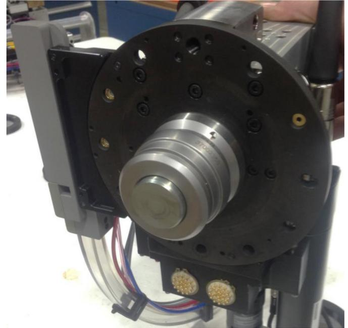
Figure 4. Tool interface with electrical, pneumatic, and fastener feed connectors.
