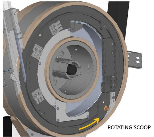
Figure 11. Fastener redirected by scoop into exit ramp.
