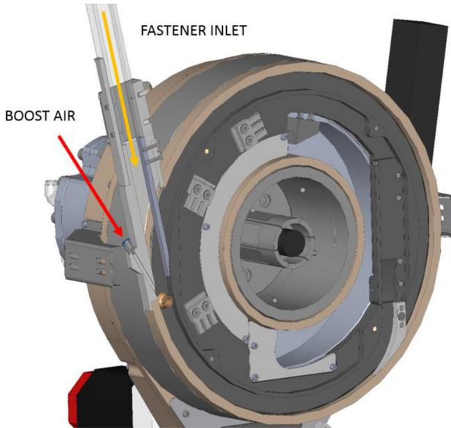
Figure 10. Fastener and airflow inlet.
