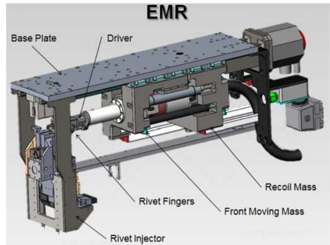
Figure 3. Electromagnetic riveter retracted
