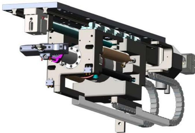
Figure 2. Electromagnetic riveter
