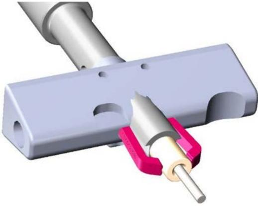
Figure 10. EMR fingers stripped back over the die
