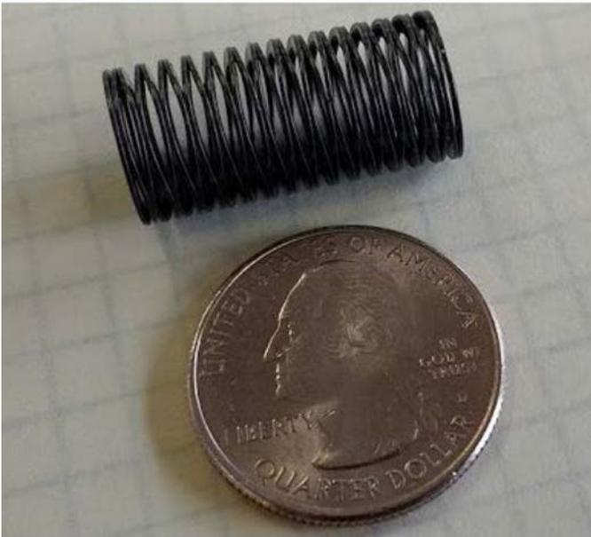
Figure 11. Wave spring pushes fingers closed
