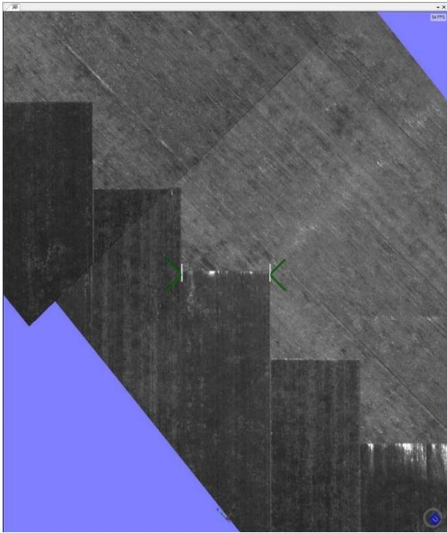
Figure 12. Semi-Automated Ply Boundary Inspection Measurement
