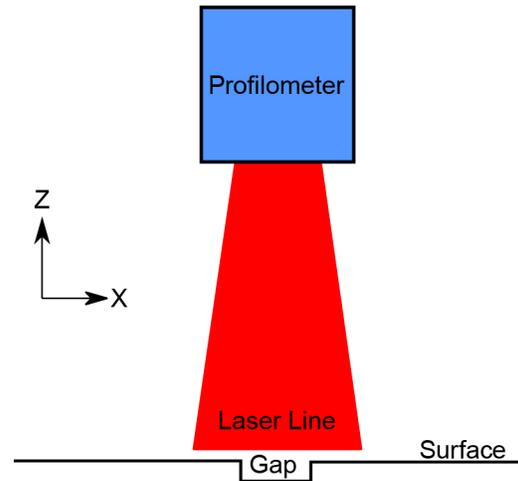
Figure 2. Profilometer Diagram
