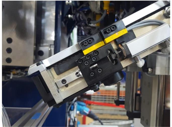
Figure 11: Air cylinder injecting rivet
