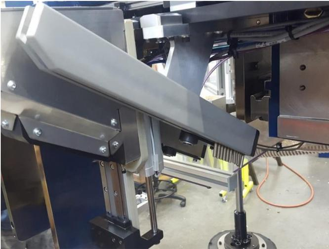
Figure 14: Hanger feeder for extremely long fasteners
