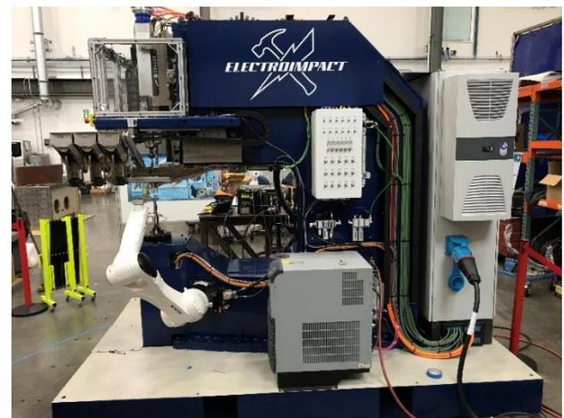
Figure 2: Flexible all electric riveter
