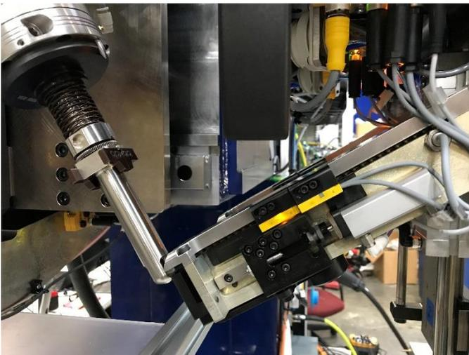
Figure 4: Air cylinder mechanism in contact with the hopper
