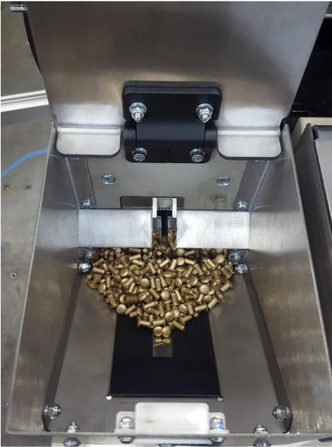
Figure 9: Flexible riveter hopper
