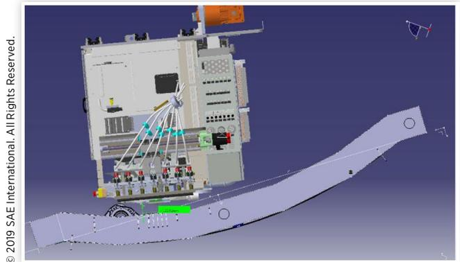
upper head 90° from its standard orientation, so that the wide direction of the head falls along the long direction of the part. This change permits the head to approach the inner skin more closely. A longer-than-normal nosepiece is still necessary, but its length is significantly shorter than would have been required without the rotation.
