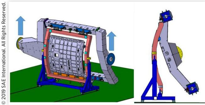
**FIGURE 4** RAJ with door after being lifted from cart by machine positioner.
