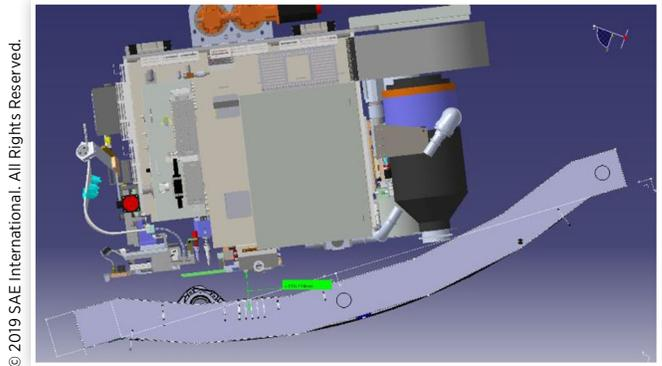
**FIGURE 6** E7000 head rotated 90° so that the narrower dimension is in the direction of panel curvature.
