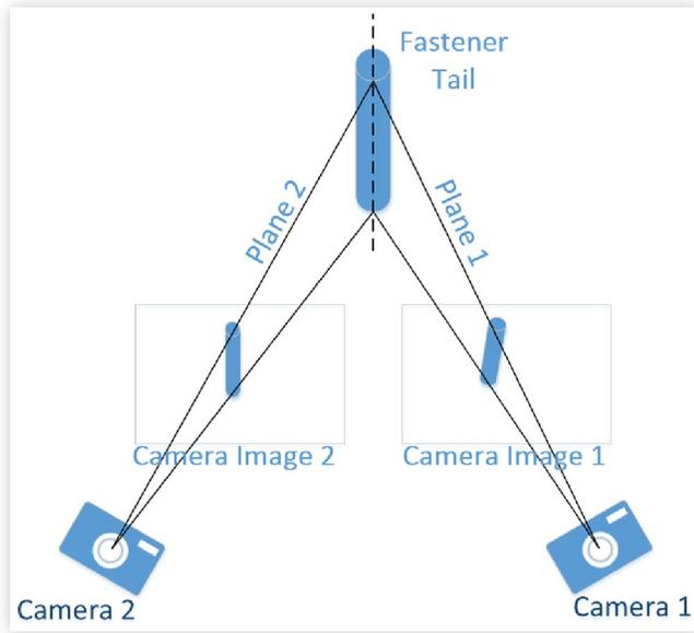
parameter. This is done for both cameras to create two intersecting planes (Figure 8). The location at which these planes intersect is the centerline of the fastener in 3D space.
