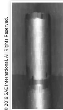
first passing a convolution kernel over the image that removes the fastener threads or ridges on a pull tail type fastener (*Figure 5, 6*).
