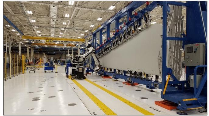
**Figure 5.** Robot system working on a rudder which is one of the larger assemblies processed by the automation
