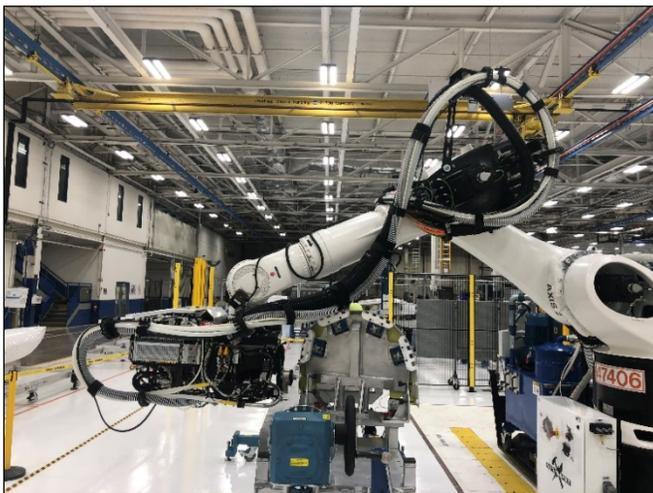
**Figure 4.** Processing a small component – in this case a fairing
