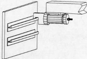
4. THE OFFSET TOOLING IS PULLED BACK TO THE STANDBY POSITION WITH AN M44. THE AERAC IS NOW CLEAR TO MOVE IN THE Y DIRECTION TO THE NEXT STRINGER.
