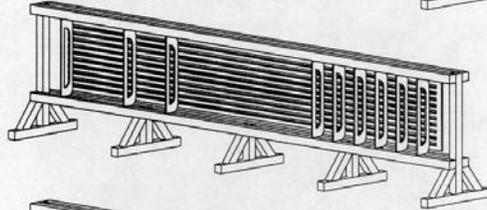
AFTER COMPLETING THE FIRST BAY, THE OPERATOR REPLACES FORMBOARDS IN THE FIRST BAY AS NEEDED AND REMOVES FORMBOARDS TO OPEN A SECOND BAY.
