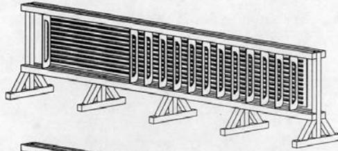
THE OPERATOR REMOVES THE FIRST SEVERAL FORMBOARDS TO OPEN UP A BAY. THE AERAC INSTALLS RIVETS ONE SIDE OF THE ALL STRINGERS BEFORE THE OFFSET TOOLING IS ROTATED AND RIVETS ARE INSTALLED ON THE OPPOSITE SIDE OF THE STRINGERS. THE END FORMBOARDS ARE NOT REMOVED ON THE AERAC SINCE THEY DO NOT OBSTRUCT ACCESS TO ANY RIVETS.
