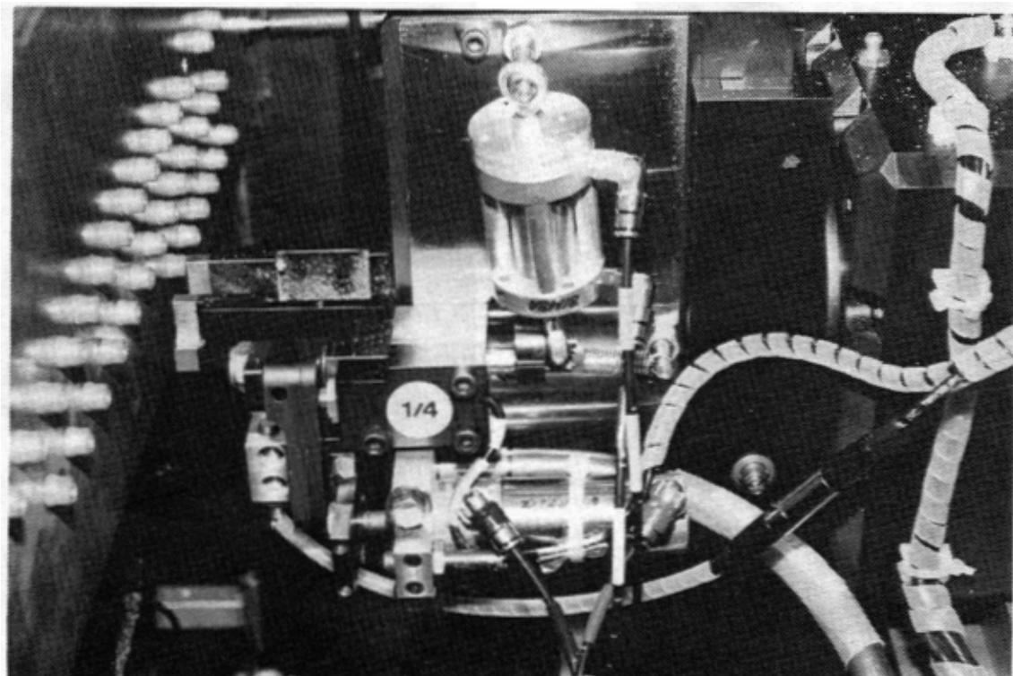
Plate 2: Collar Loading/Swaging Tooling
