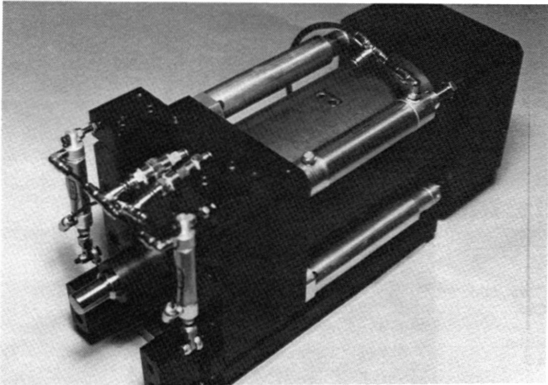
Plate 1: Low Voltage Electromagnetic Bolt Driver
