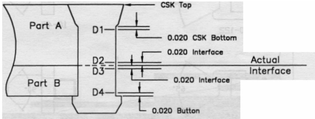
Figure 4: Location of rivet interference measurement
