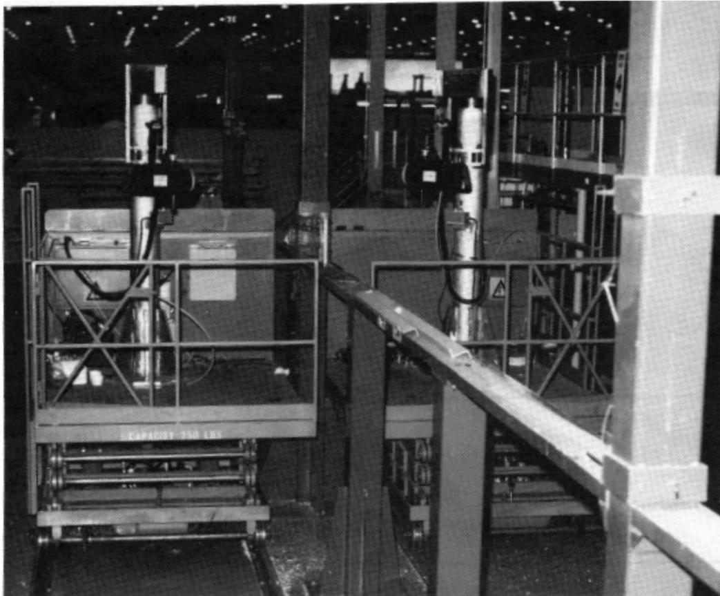
Plate 2: Unloaded Floor Assembly Station with Scissors Lifts
