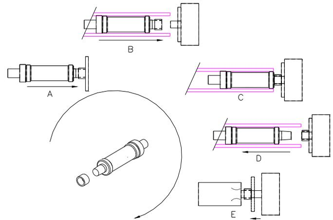
**Figure 12. Collar and Nut Feed System**
