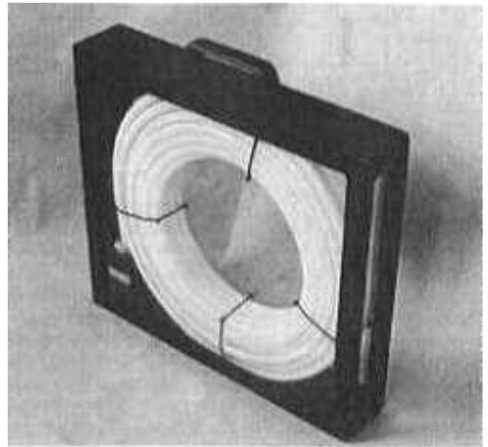
**Figure 5. Coiled Tube Magazine (Cassette)**
