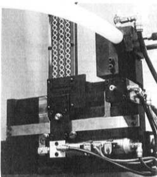
**Figure 11. Collar and Nut Feed System**
