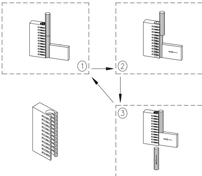
**Figure 7. Slug Rivet Escapement**
