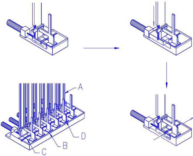
**Figure 10. Slug Rivet Feed System**
