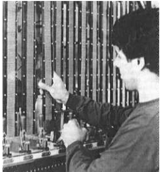
**Figure 9. Slug Rivet Feed System**
