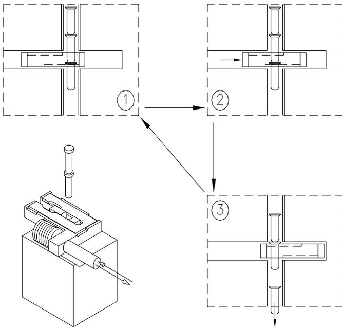
**Figure 6. Headed Fastener Escapement**
