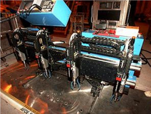
The machine frame and the drill carrying "wings" were 100% re-designed for stiffness and long term dimensional stability while reducing the front-to-back dimension of the AFDE to allow it to be loaded in through the 737 passenger doors. In addition, Electroimpact explained and Boeing recognized that some of the weight constraints imposed on the older AFDEs were somewhat artificial and that a heavier AFDE could be a stiffer, more accurate AFDE.
