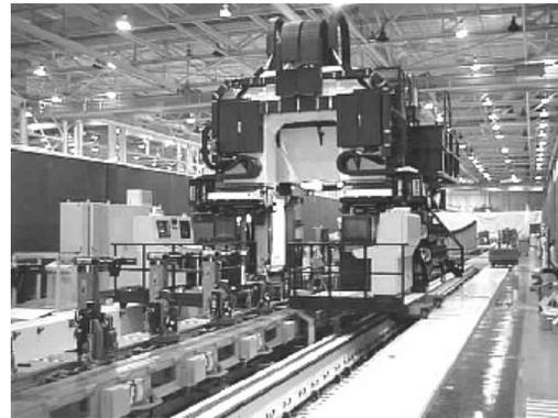
Figure 6: Loading Spar into Fixture
