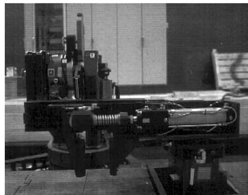
Figure 9: Upper Index Assembly with Post Fully Down
