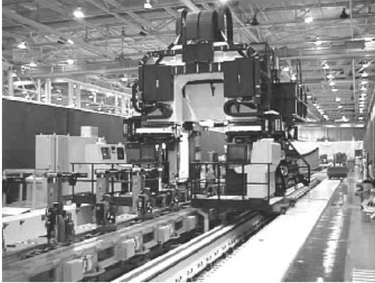
Figure 7: Spar Loaded in Fixture
