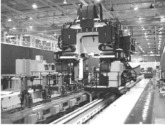
Figure 4: Fastener Feed System
