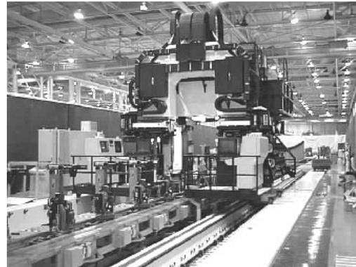
Figure 2: Clamp Table with Process Tools
