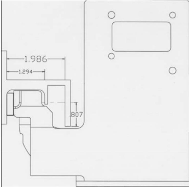
Figure 11: Anvil inside of offset stringer
