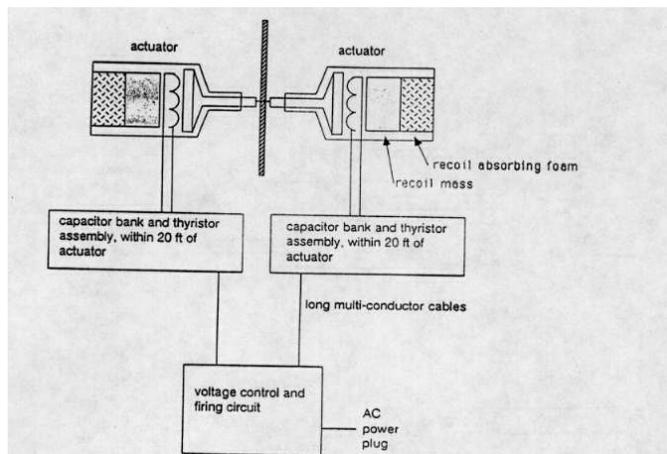
Figure 1: LVER Block Diagram
