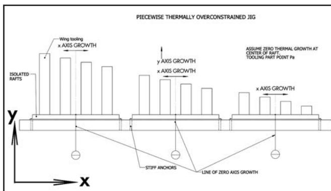
Figure 2. Simplified illustration of a piecewise thermally overconstrained jig
