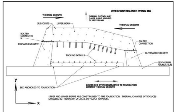
Figure 3. Thermally overconstrained jig
