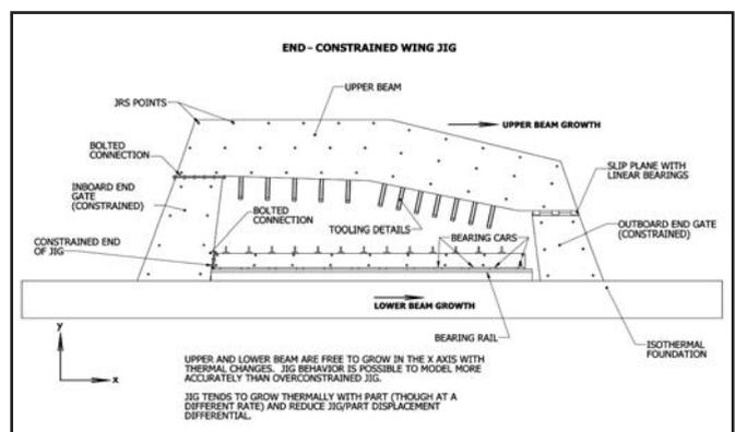
Figure 4. End-constrained wing jig
