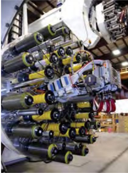
**Figure 5.** An Electroimpact AFP head, similar to the one now being used at Spirit AeroStructures to create the Boeing 787 fuselage section 41. (Image courtesy of Electroimpact)
