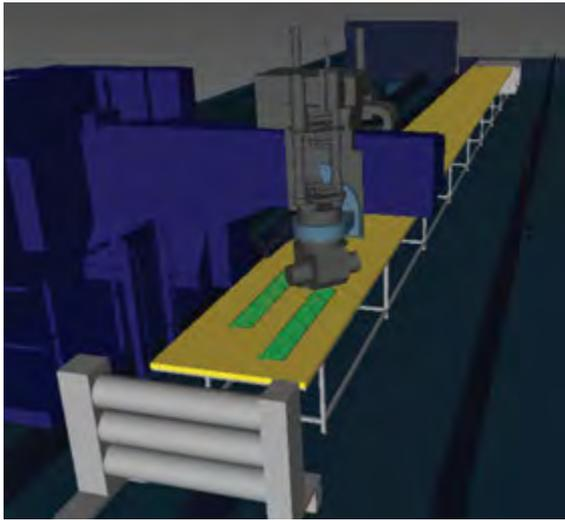
**Figure 9.** A simulation of a M-Torres AFP machine being used for wing stringer charge lay-up.
