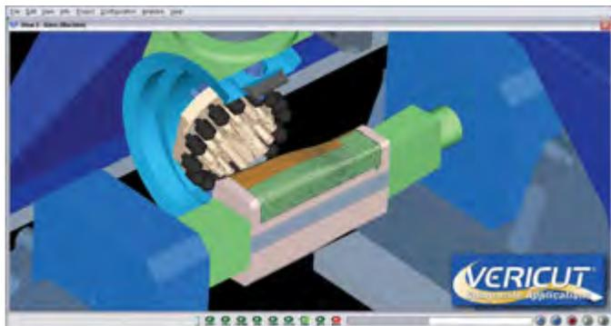
**Figure 7.** Current programming and simulation project involving an Electroimpact gantry design with removable rotisserie.
