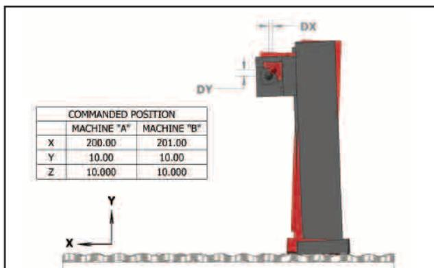
**Figure 1.** Slight variations in machine rail cause X, Y, and Z axis errors when moving in X (Illustrated by Ben Todd)
