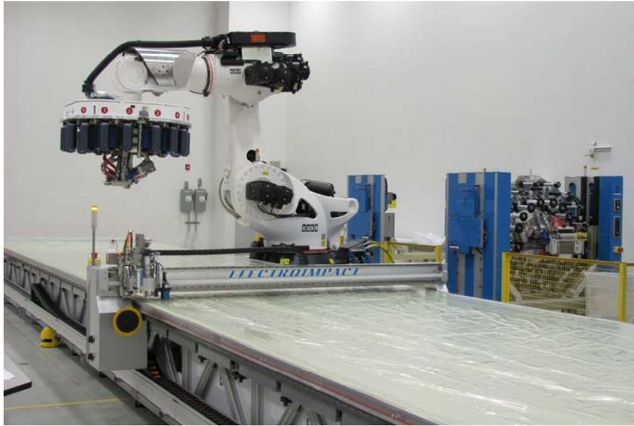
Figure 11. Robotic AFP cell with vacuum table, ultrasonic cutting gantry, 2 AFP heads (1/4" and 1/2"), and head changing stands.
