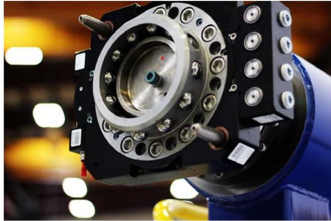
Figure 2. Robotic tool changer utilized for quick-change AFP heads
