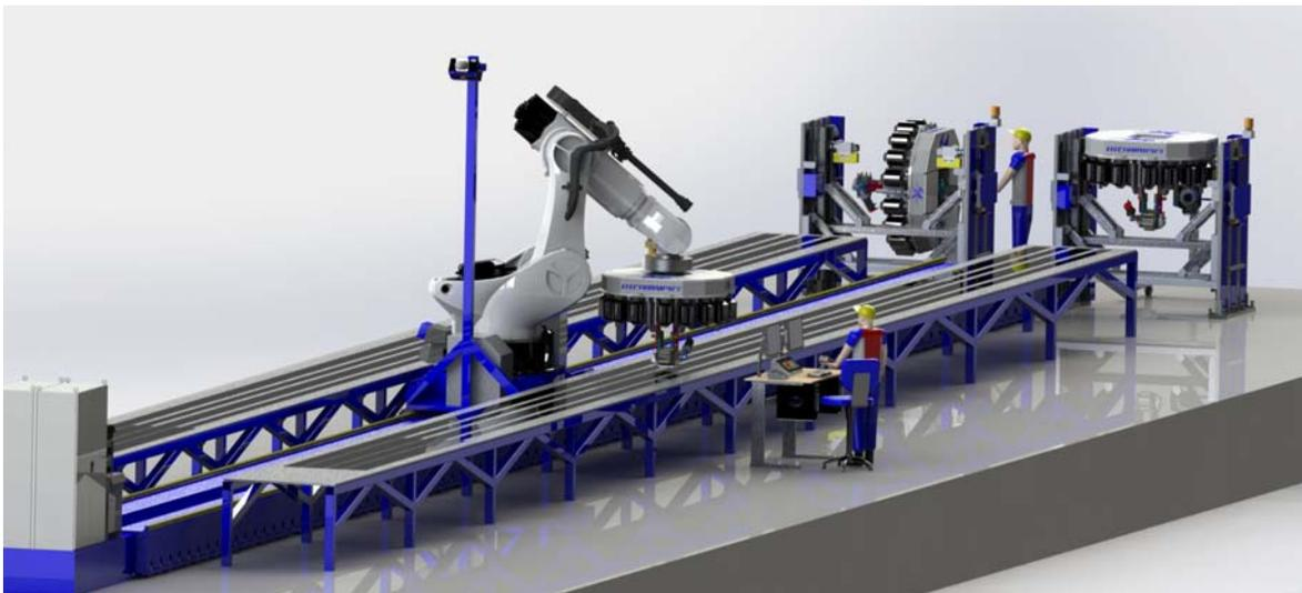
Figure 14. Robotic AFP stringer charge cell with two vacuum tables, ultrasonic cutting head, head change stands, and laser projection.
