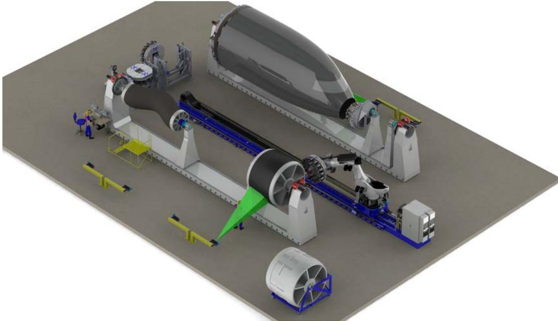
Figure 13. Robotic AFP cell with multiple rotators, head change stands, and laser projection.
