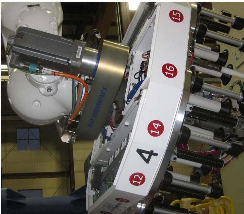
Figure 6. Axis 6 with modular Electroimpact AFP process head.
