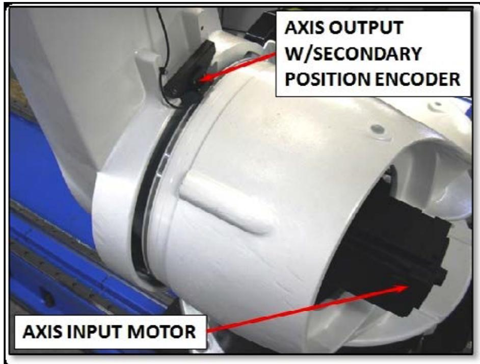
Figure 1. Industrial robot axis with secondary feedback installed.
