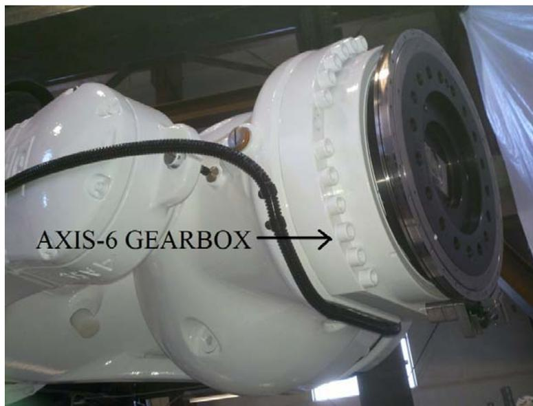
Figure 4. Standard Kuka Titan Axis-6
