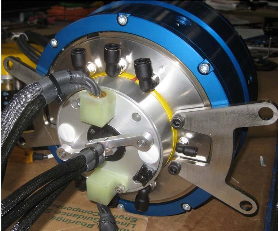
Figure 7. Pneumatic rotary union with power and signal slip-rings.
